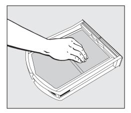
Use your fingers to remove the fluff from the surface of the filter. Remove any fluff from the hollow part of the door holder. A cleaning brush is available as an optional extra from your Miele dealer or the Miele Spare Parts Department.
